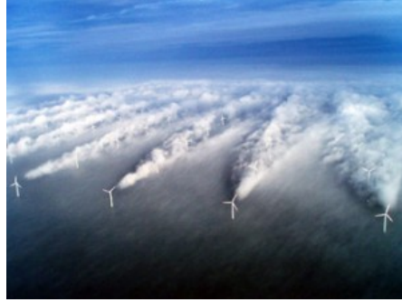
Fig 1: Illustration of wake effects (excerpted from Zwakman (2014))
