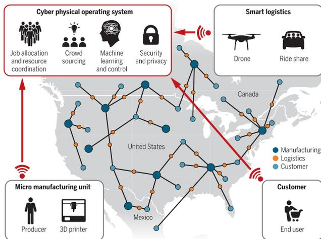
**FIGURE 13.** Cyber-physical operating system connecting and coordinating customers, micro-manufacturing units and smart logistics to enable massively distributed manufacturing. Reprinted from C Okwudire and H Madhyastha, *Science* 372, 341 (2021); Graphic: C. Bickel.
